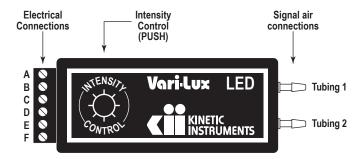
A: 5 VDC positive (+) C: Tubing 1 positive (wht +) E: Tubing 2 positive (wht +) B: 5VDC negative (-) D: Tubing 1 negative (blk -) F: Tubing 2 negative (blk -)
